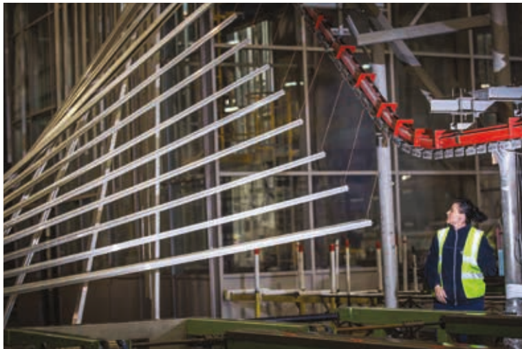
Left The automated vertical powder-coating line lifting the aluminium profile lengths through pre-treatment, powder-coating and baking processes.
