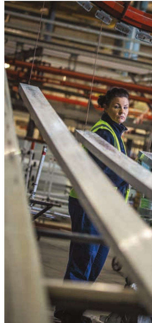
Left The automated vertical powder-coating line lifting the aluminium profile lengths through pre-treatment, powder-coating and baking processes.
