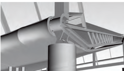
Detail at column/bullnose/rooflight interface
