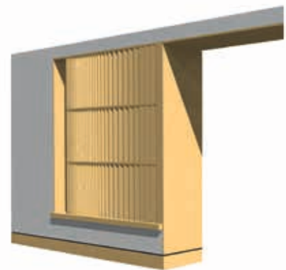
BELOW: Visualisation and plan image of the stone louvred screen that forms part of the rear extension elevation, allowing passive ventilation strategies to be securely applied.
