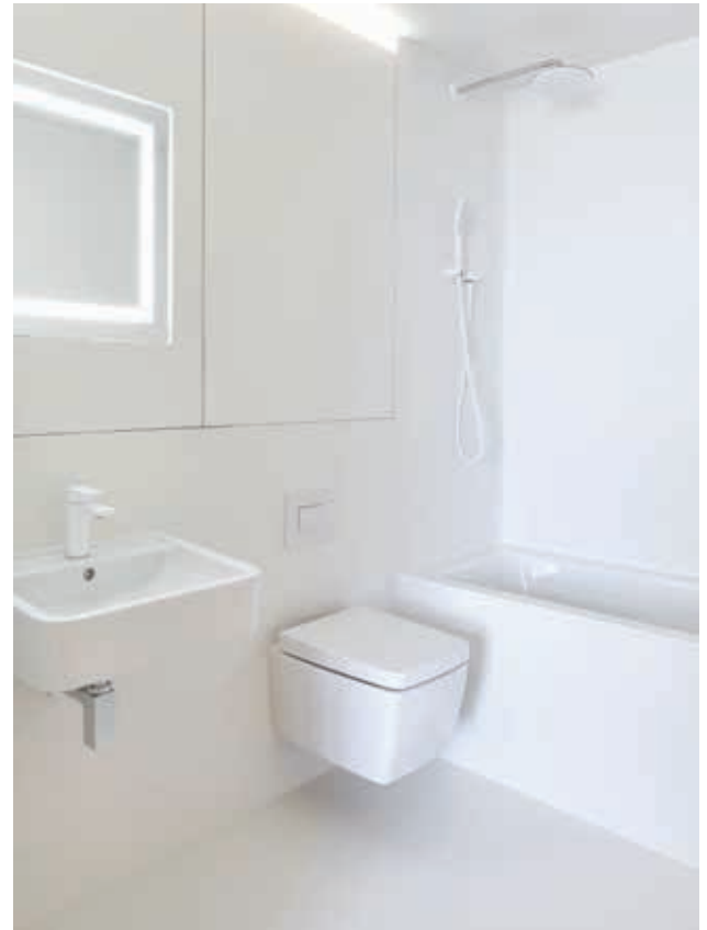
At Amin Taha and Groupwork's Barratts Grove housing, the rich, warm, timber cladding outside the bathroom is counter pointed by 2001-like stark whiteness within – tile free to cope with structural movement.
