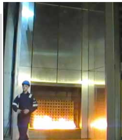
Above BS 8414 large-scale system test on Kingspan's insulated wall liner panel with aluminium hook-on cassette
