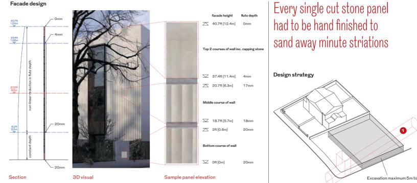
'The machinery and blades needed to be in perfect condition,' says McConnell. 'We had to make metal templates of the top and bottom of each stone panel to ensure flute sizes were going to align on consecutive panels.' File sizes for the 3D model were huge, he recalls. 'Towards the top we were working with cutting radii of 1.8km.'
