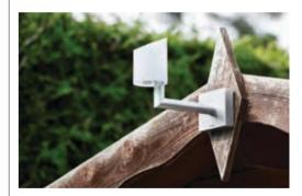
**Above** Gira weather station. Wind speed, precipitation, twilight and temperature can be measured and analysed with the new KNX weather station Standard. **Below** Thornby is a traditional brick house with parkland.
