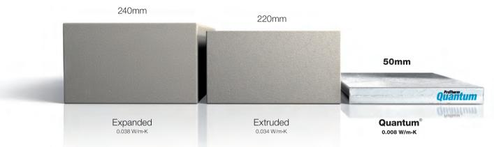
The depth of board to achieve an R-value of 6.250 m<sup>2</sup>K/W – rounded up to the nearest standard depth.
