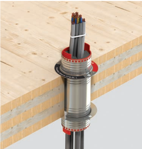
Right Brockett outlined various means that Hilti had employed, such as the CFS-SL sleeve and CFS-CC collar, to mitigate the potential fire effects on solid CLT construction.
