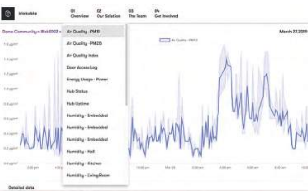
Above The BlokSense Insights Dashboard is pre-installed in a hardwired system built into the Blokable Building System, equipping community and property managers with software tools to monitor safety and performance, manage access, and improve comfort.
