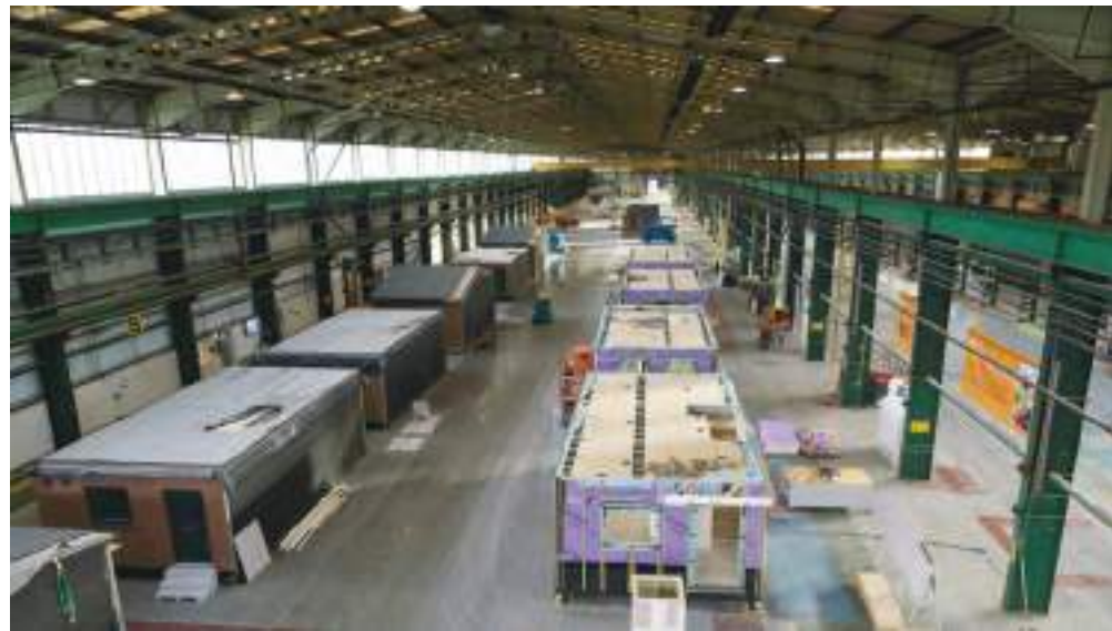
Above Modules on the production line at the Ilke Homes factory in Knaresborough, North Yorkshire: safer, quicker, cleaner, more sustainable. Left Architecture as product design: a module being craned into Ilke Homes' Hawthorne Avenue development in Hull.
