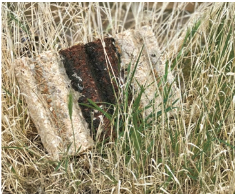
Above WoWood is a new product made from waste sawdust and carrageenan natural binder. Below It could be used for acoustic panels, even partition walls. Early tests show it is easily reshapable.
