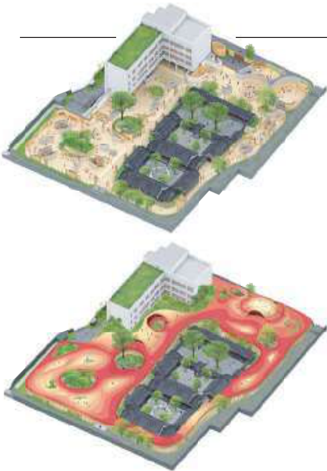
Left Ground floor and roof axonometric. Ground floor spaces flow into each other, abandoning the idea of traditional classrooms.
