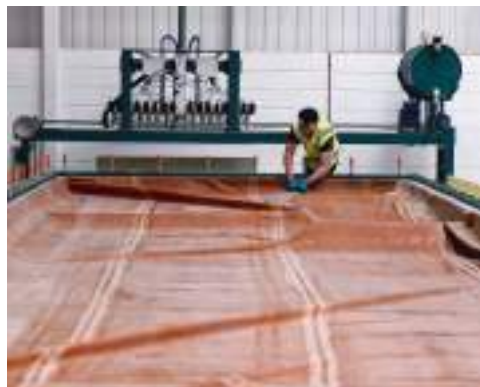
Left The COP26 demonstrator is being constructed at CSIC's specialist facility using the only vacuum press of its kind in the UK.
