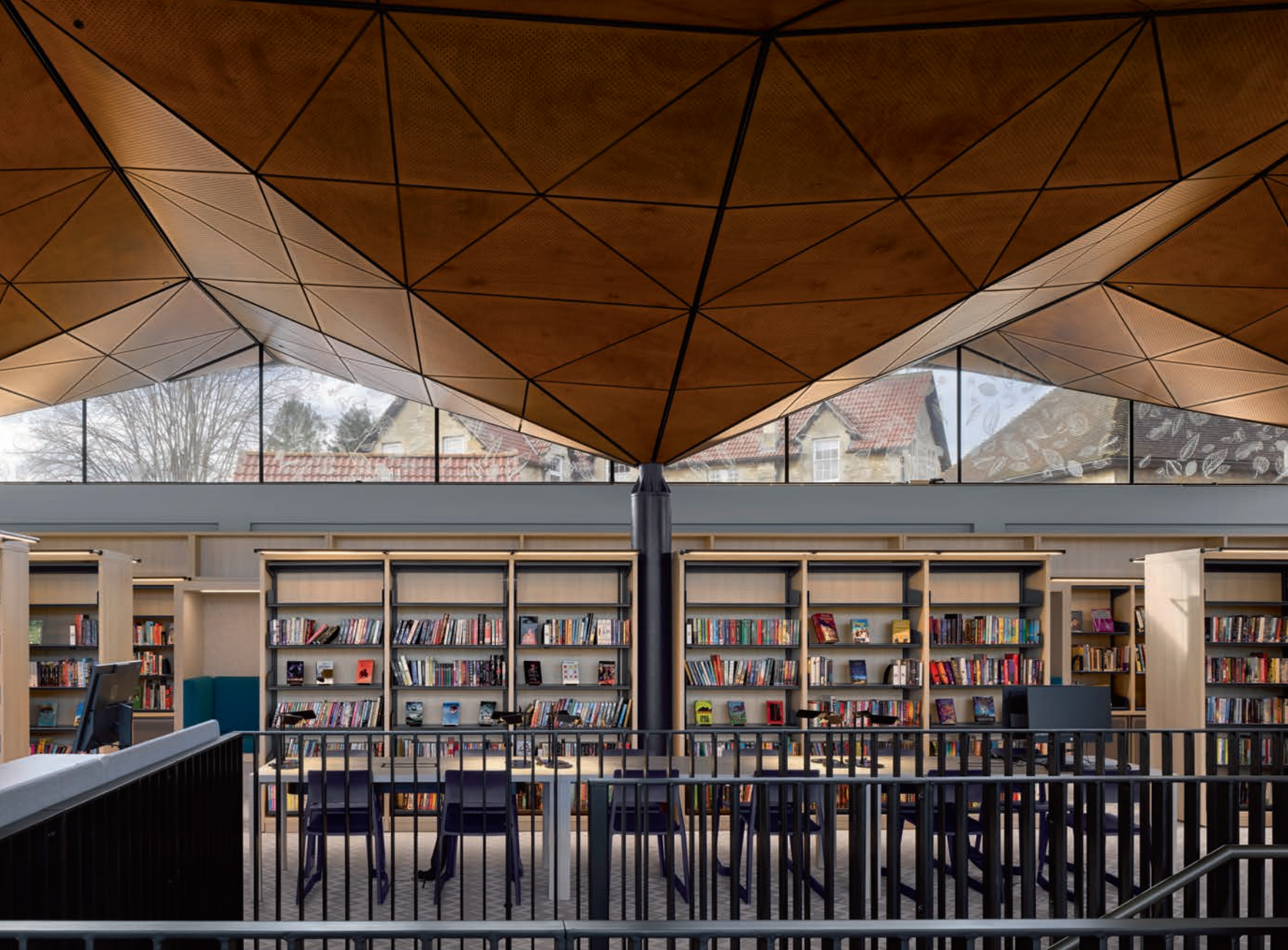
Above The roof is raised up on steel ‘trees’ giving a clerestory right around the first floor (as diagram, below).
