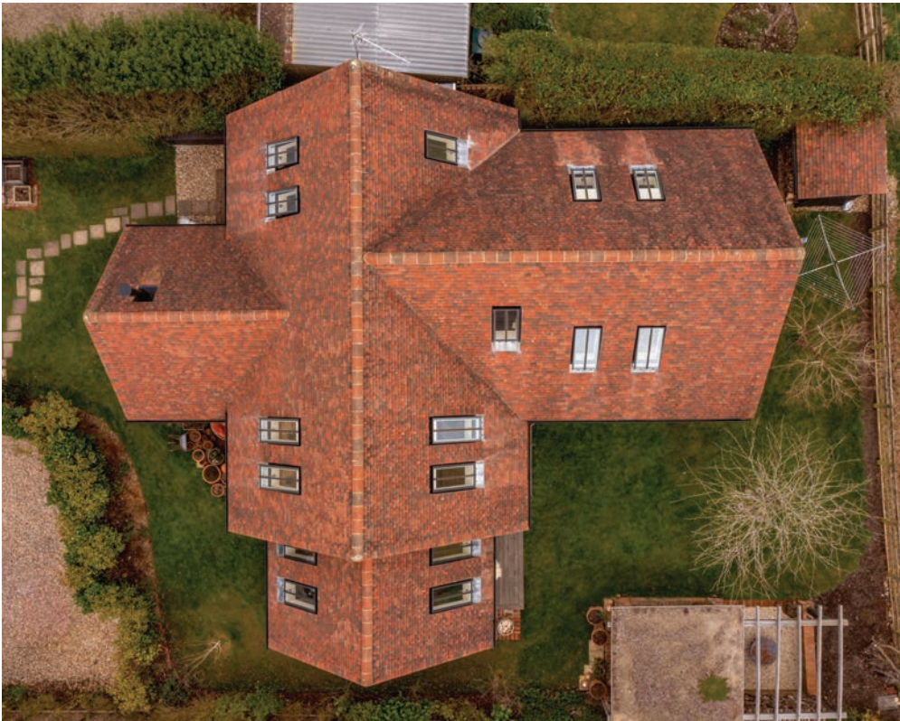
Above Adding rooflights meant extra rooms could be added to the eaves of the property.
