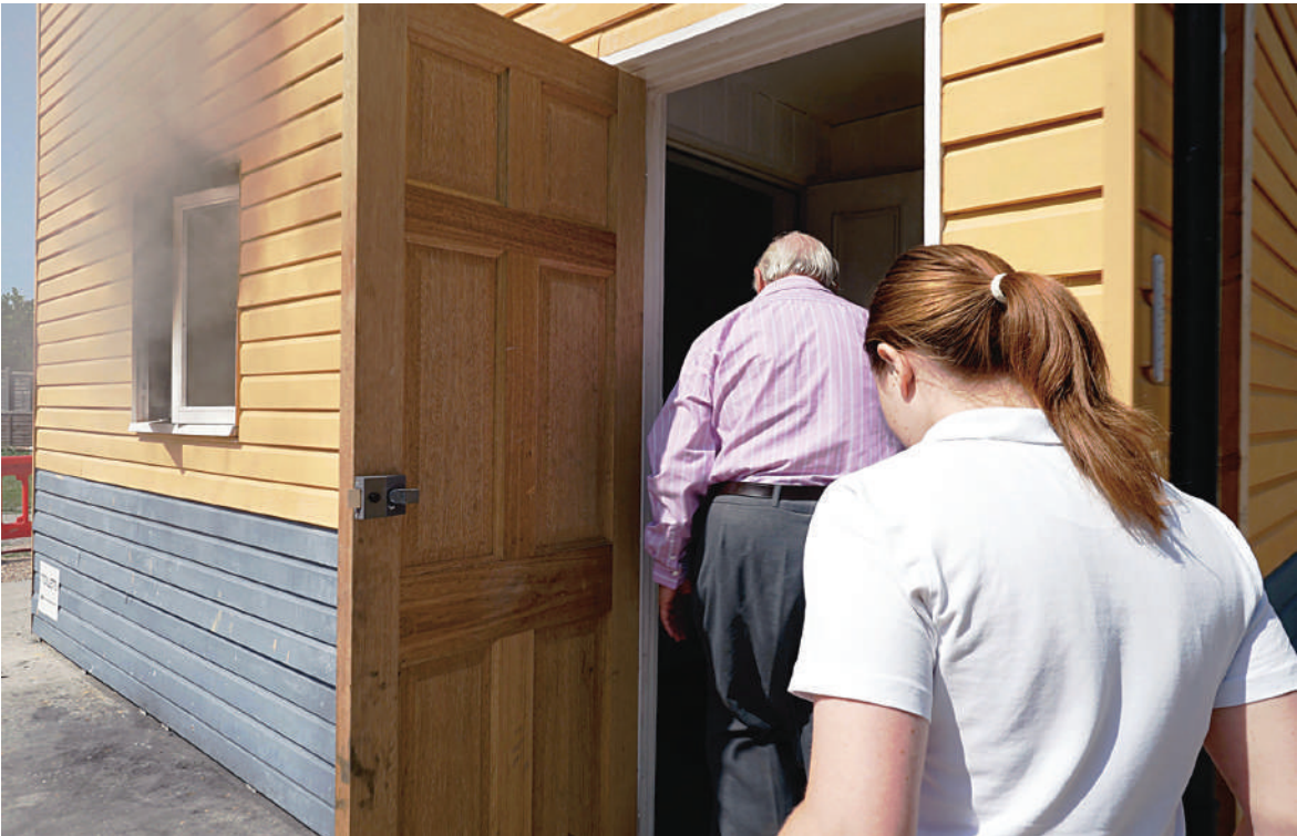
Above A fully furnished test house was constructed and fires set on both floors. Architects, engineers, surveyors and the NHBC were among those observing the house during the fire.
