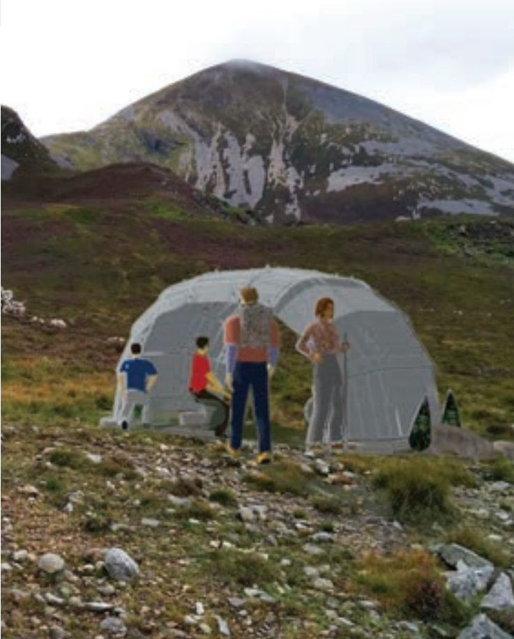
Above The shelter is a quasi-permanent structure made from galvanized steel panels
