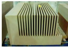
Above A typical process for stone corner quoins can lead to considerable material wastage. Could this be formed of two flat slabs by introducing a joint to reduce waste?
