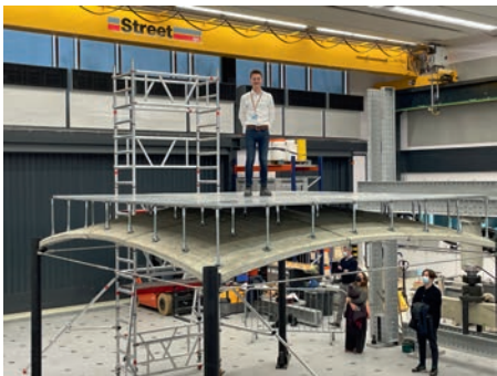
Above A prototype ‘thin shell’ vaulted floor slab, developed by an interdisciplinary team from the Universities of Bath, Cambridge and Dundee, generates 60% less embodied carbon than the equivalent flat slab.
