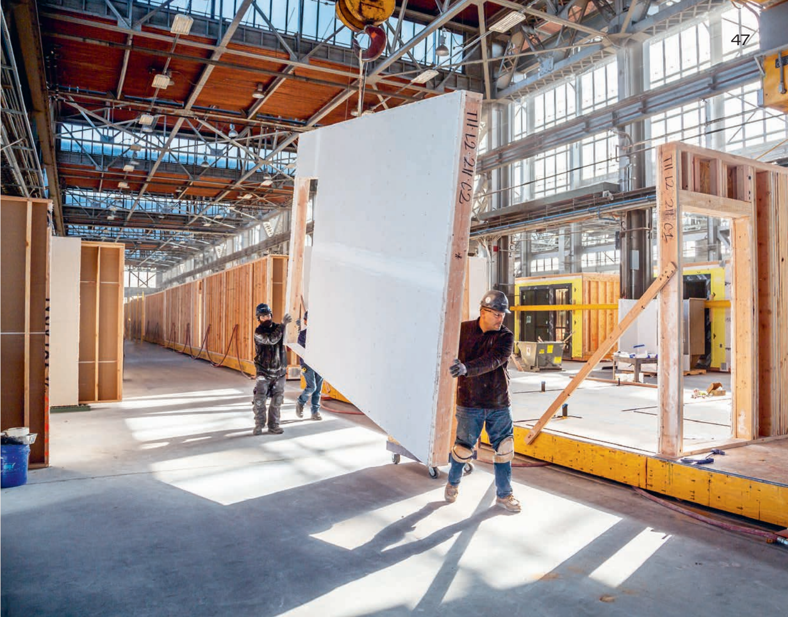
Above Employees at construction-technology company Factory_OS in Vallejo, California, assemble modular homes at the company's warehouse.
