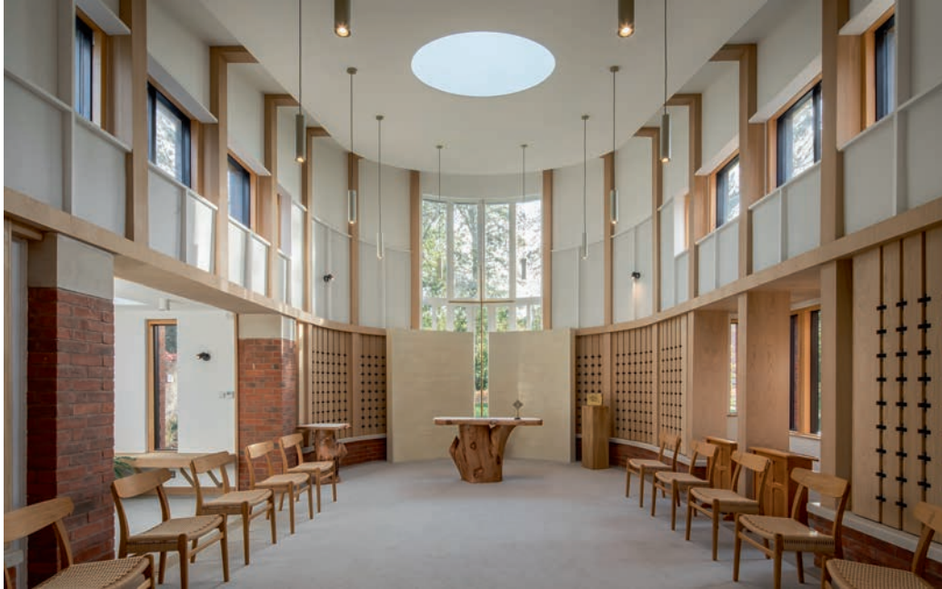
Above The chapel interior has acoustically absorbent perforated timber panelling.
