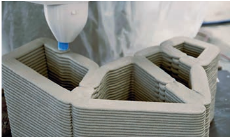
Top The 104 hollow 3D printed concrete pieces of Phoenix work solely in compression so it is easily assembled and disassembled.
